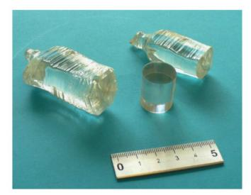
Fig. 2.3. Photo of the  $ZnMoO_4$  scintillator and crystal boules produced in Nikolaev Institute of Inorganic Chemistry by the low-thermal-gradient Czochralski technique. The scale is in centimeters.
