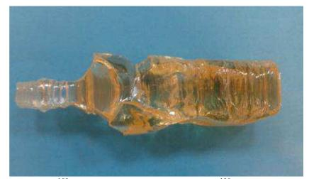
Fig. 2.7. Photo of the  $Zn^{100}MoO_4$  crystal boule enriched in  $^{100}Mo$  to 99.5%. The boule with the mass of 170.7 g and length of 95 mm was grown for the first time by using low-thermal-gradient Czochralski technique in the Nikolaev Institute of Inorganic Chemistry.
