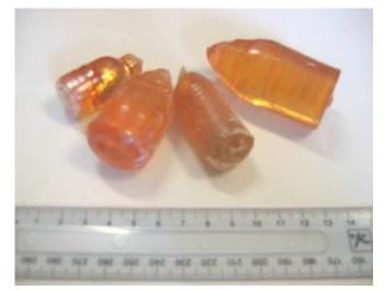
Fig. 2.2. Photo of the  $ZnMoO_4$  crystals 20 mm–30 mm in diameter and 30 mm–40 mm in height grown by the Czochralski technique in 2009 year [158]. The scale is in centimeters.
