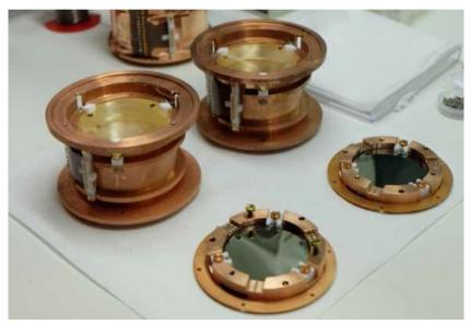
Fig. 2.17. Photo of the scintillating bolometers based on 336 g and 334 g  $ZnMoO_4$  crystals of advanced quality with their ultrapure Ge photodetectors.
